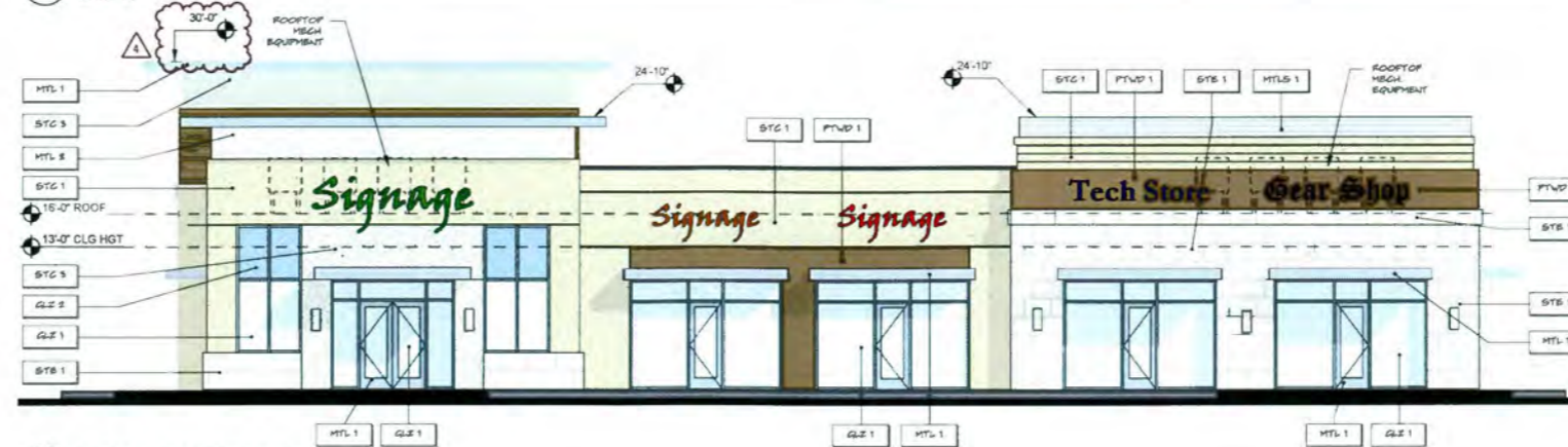
4 L-WEST ELEVATION (BUILDING M EAST ELEVATION) Scale: 1/8" = 1'-0"
