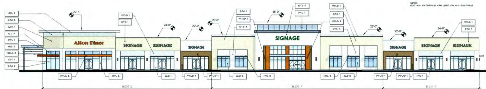
1 EXTERIOR ELEVATION - NORTH Scale: 1/16" = 1'-0"
